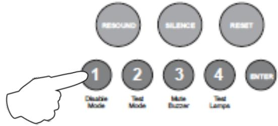
Pressing the Disable Mode button again will move disable selection mode to Zone 2 and the Zone 2 Fault/Disabled/Test LED will be pulsing instead. Subsequent presses will move the selection to Zones 3 - 12, dependant on the number of zones fitted to the panel. I.e up to zone 4 on a 4 zone, 6 on a 6 zone, 8 on a 8 zone etc.
