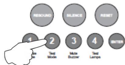
When finished, press and hold Button 1 for 3 seconds to save setting and exit programming mode.
