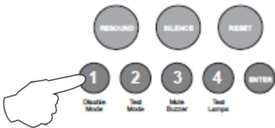
Use button 1 to scroll to the function that requires editing for that output, indicated by a pulsing fire LED 1 - 5 as per table below.
