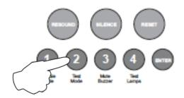
With the required zone LED lit, press the ENTER button to enter 'edit mode'. The fire LED will now pulse. Now use button 2 to turn on delays, this is indicated by the zone, amber, fault / disabled / test LED, ON.
