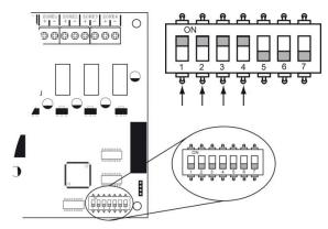
To set Twin Wire mode for zones A-D on the zone extension circuit boards, move switches A-D on the 4 way DIL switch located on the zone card to the 'ON' position.
