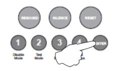
When all zones to be tested have been set, press and hold the Test Mode button for 3 seconds again. This will exit the test selection mode. All zones in test and the Test Mode will now be indicated by a steady LED.
