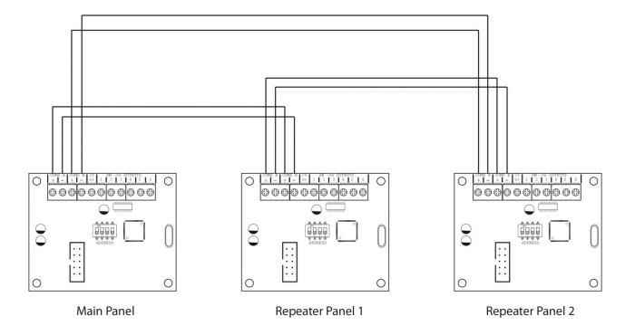
When finished all panel wide programming, enter the next programming code or disable the controls and return DIL switch 6 to 'OFF'.
