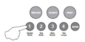
Now use button 1 to move the pulsing fire LED to the required setting as per the table below, then use button 2 to select the function.
