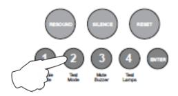
During viewing it is possible to delete the entire history by pressing and holding button 2. The panel will chirp to acknowledge deletion.
