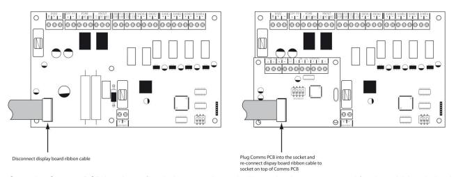
Once the Comms PCB has been fitted, the control panel will need to be programmed for the additional circuit board. See panel wide settings 2-1-2-3 option 5 (Setup Internal PCB Configuration) on page 26.
