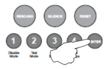
Press the ENTER button to return back to the zone selection, indicated by a steady zone fire LED
