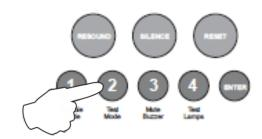
Pressing button 2 again will toggle the compatibility mode on & off, indicated by the zone 1 Fault/Disabled/Test LED.
