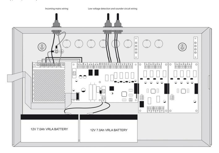
Drawing shows typical internal layout of the panel cabinet with two 3.2Ah, 12v batteries fitted
