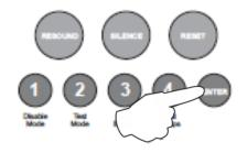
Press the ENTER button to enter 'edit mode' and zone 3 fire LED will pulse.
