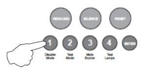
Pressing the Disable Mode button again will move disable selection mode to Zone 2 and the Zone 2 Fault/Disabled/Test LED will be pulsing instead. Subsequent presses will move the selection to Zones 3 - 12, dependant on the number of zones fitted to the panel. I.e up to zone 4 on a 4 zone, 6 on a 6 zone, 8 on a 8 zone etc.
