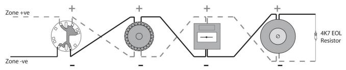
Twin Wire systems require special 'sav-wire' detector bases and polarised call points but standard sounders. Most modern, non-addressable, low current, polarised sounders, bells and beacons are compatible, Cooper Fulleon, Besson, Klaxon etc.
