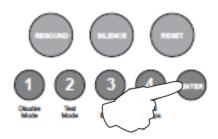
When the end of the log is reached the panel will drop out of view mode.
