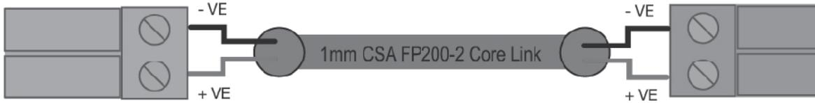
Line - Connector on Network / Compact unit to black phone lead
