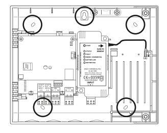
Note: the supplied back box mounting template can be used to drill the fixing positions, if required.
