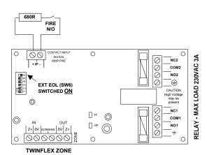
For use as an unmonitored input, connect to input as shown above, remembering to set the External EOL switch to ON.
