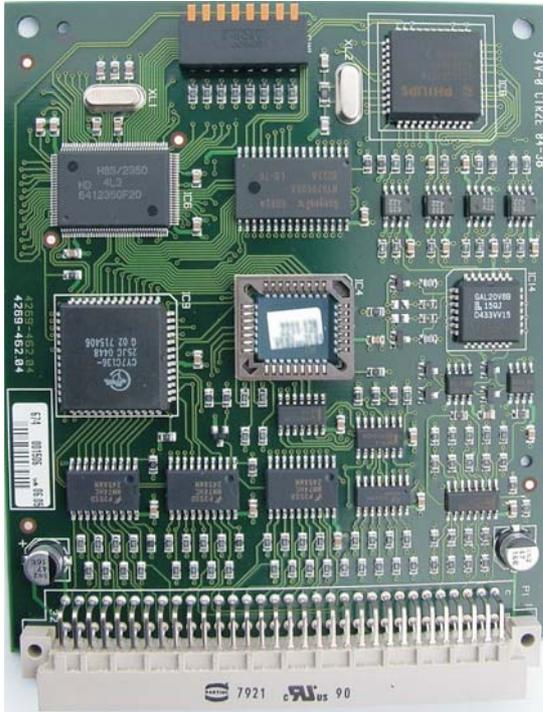
This copper network card is used to allow data to pass between control panels and network nodes installed in a networked fire system. The card must be plugged into the backplane of the panel or node in a dedicated slot. When it is plugged into the slot P8 on the backplane the external cables must be connected to terminal block P10, which is also on the backplane.
