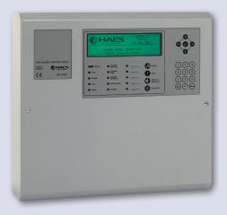
The HS-4100S comes fitted complete with an internal loop driver card suitable for Apollo (XP95 & Discovery) and Hochiki (ESP) protocols and 2 on-board sounder circuits.
