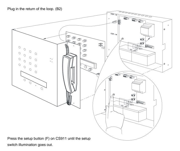
The front control panel will sound twice to signify that the system has come out of the setup mode.
