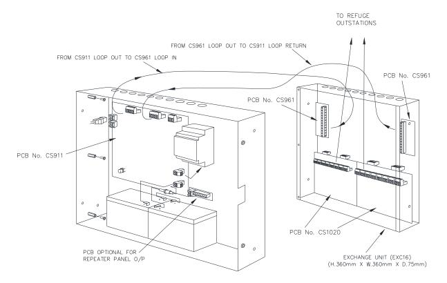
The EXC8 exchange PCB CS1020 has a set address on the loop. The output numbers will depend upon the address SW1 switch as below :
