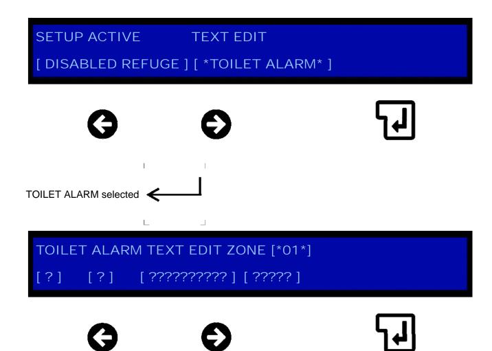
Pressing the right or left buttons allows the toilet alarm zone number to change to the desired text location to edit. As the system is in setup the responding or active remote outstations will be displaying on the 1-16 zone buttons above the LCD screen. These same zone numbers refer to the text locations required for each zone for each toilet that is wired to its local refuge point.
