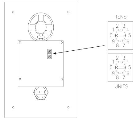
The remote outstation address is SW1 Tens and SW2 Units
