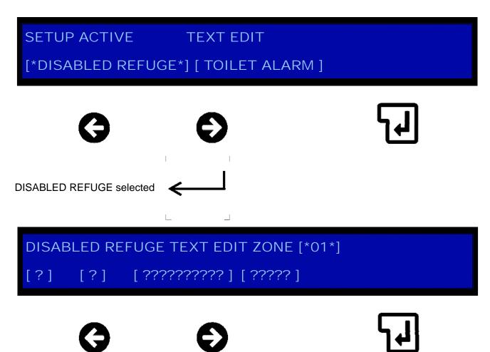
Pressing the right or left buttons allows the disabled refuge zone number to change to the desired text location to edit. As the system is in setup the responding or active remote outstations will be displaying on the 1-16 zone buttons above the LCD screen. These same zone numbers refer to the text locations required for each zone.
