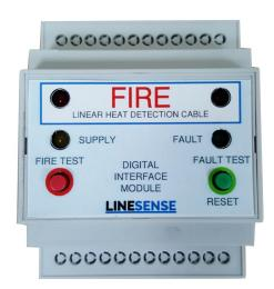
The Digital Interface Module (DIM) monitors the Linear Heat Detection (LHD) cable for both Fire and Fault (open circuit) conditions. By the use of an additional series resistor it can also offer discrimination of a short circuit fault on the interposing field wiring.
