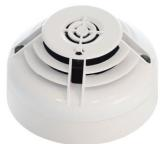
The sensing elements of the SMART3 are panel controllable so the sensitivity thresholds of each element can be changed by the panel offering the ability to customise the device for the changing use of the area it is protecting. The detector has built in short circuit isolation and two integral tri-colour LEDs that provide 360° local visual indication of the device status. The LEDs are programmable with static or blinking red, amber and green status indications available.
