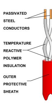
LHDC Digital may be used as a simple switch to operate a relay etc. However in most installations the minimum requirement is that the LHDC circuit is monitored for disconnections by means of EOL device and an appropriate fire alarm channel or address loop interface unit.
