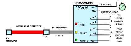
Figure 2 shows a simple configuration with the unit directly connected to a fire panel trigger
