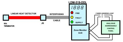
Notes: Configurations for Fig 2 & 3, is dependant on the voltage and current specifications of the LDM-519-LP being compatible with the monitoring technique and electrical characteristics of the Control Panel / Zone Monitor Unit.
