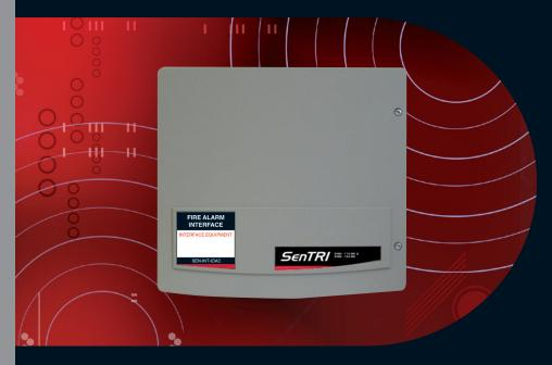
The new SenTRI Mains Switching Interface units connect directly to the loop of SenTRI 2 and 4 loop systems. The interface units are designed to provide heavy duty relay switching for both 24V and 230V applications with contacts rated at 13A. This interface is particularly suitable for switching damper control units and other building controls requiring a high contact rating for mains shutdown.
