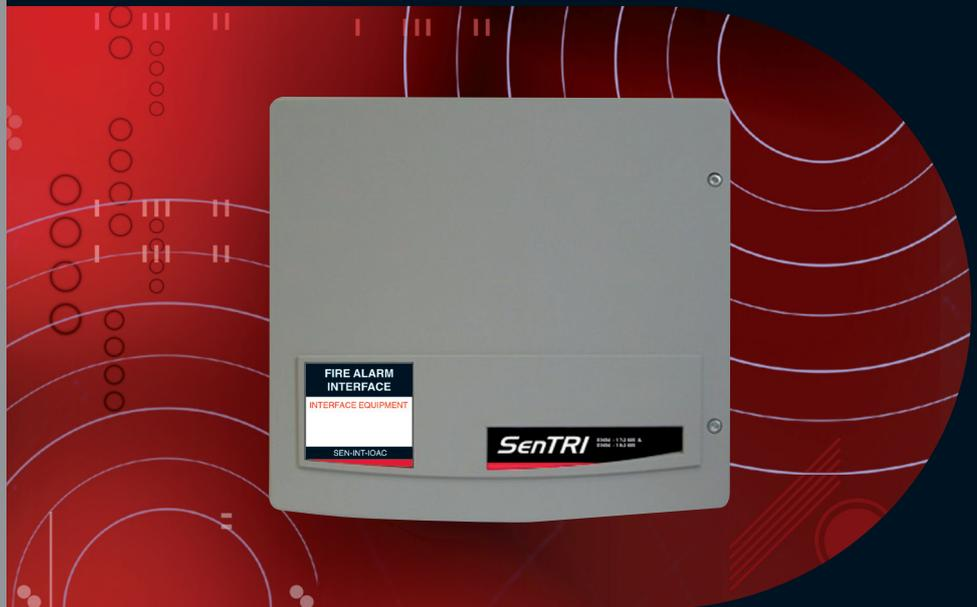
The new SenTRI Mains Switching Interface units connect directly to the loop of SenTRI 2 and 4 loop systems. The interface units are designed to provide heavy duty relay switching for both 24V and 230V applications with contacts rated at 13A. This interface is particularly suitable for switching damper control units and other building controls requiring a high contact rating for mains shutdown.
