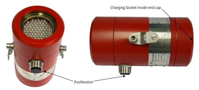
The picture above shows the FS301 flame simulator. The on/off pushbutton is shown to the underside of the flame simulator. The charging socket is on the reverse end from the faceplate window, inside the end cap. The FS301 flame simulator will operate for a maximum of 60 seconds before timing out.
