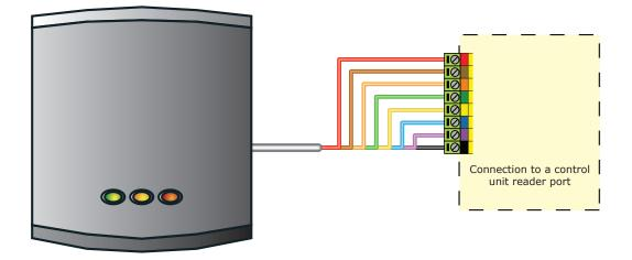
WHITE labelled control units provide 5V at the Red terminal. The Red power wire for the reader should therefore be directly connected to the 12V supply terminal.
