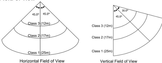
To comply with the directional dependence requirements for EN 54-10:2002 an angle of ±30° from 0° (0° = Orientation of detector in same axes as flame source) should not be exceeded, based on lab testing at a distance of approximately 5.0 ft (1.5 m).
