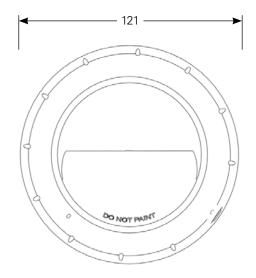
NOTIFIER by Honeywell's EN54-23 approved Wall Mount Sounder Strobe integrates a 32 tone sounder and high-quality strobe into one device. It is powered by the fire panel via the loop wiring. Operation and control of the device is via Notifier OPAL Protocol or CLIP Protocol. The device is installed simply by a twist fit onto the universal B501AP base.
