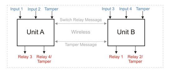
The Wireless Relay system has many applications where short range transmission of simple switches is required, for example, PA buttons, door contacts, remote sounders, lighting, door locking etc. The units are supplied in double gang plastic plates.
