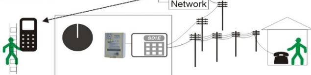
If an auto-dialler SD1E is used for communication as in scenario 3 then it is possible to use the communication link to enable the worker to use a mobile phone to generate an OK signal to restart the countdown timer. This would enable say a patrolling security guard to cover a large site without the need for dozens of hardwired OK/AV acknowledge buttons. Optional OK/AV buttons can be used if necessary to enable the countdown timer to be reset.
