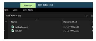
On the computer, the TalentumTT<sup>2</sup> will present itself as a read-only USB drive containing two files, *calibrations.csv*, and *tests.csv*.
