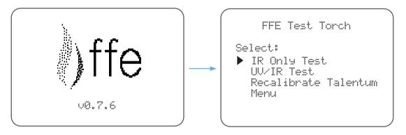
Whilst the unit is powering up, the battery will be checked before taking you to the main screen.
