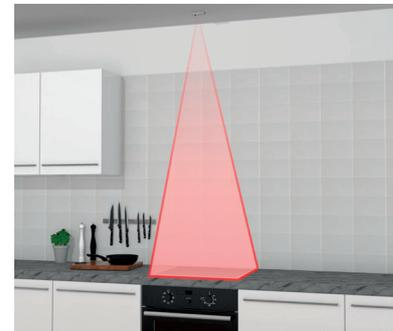
For ceiling installations, the supplied IR lens extension must also be fitted. See page 11-12.
